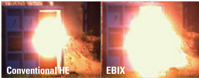
Comparison of blast effect between conventional HE and EBIX ammunition
