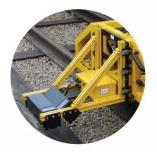
Measure 3rd rail alignment profile using laser technology
