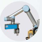
Detect bolt cracks using ultrasound technology
