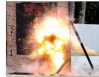
Blast effects of HE cartridge
