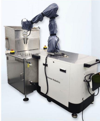
Underwater Nanobubble Airfoil Polishing Cobot
