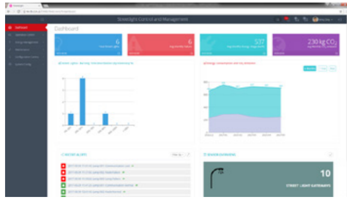
Dashboard view with alert notification, power consumption graph and lighting status
