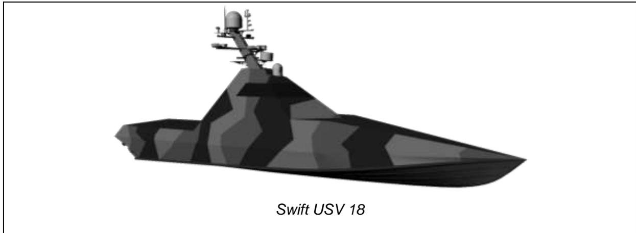
The Swift USV is a variant derived from the proven “Deep-Vee” planing hull form, which can be enhanced by integrating an air cavity on the underside of the hull.
