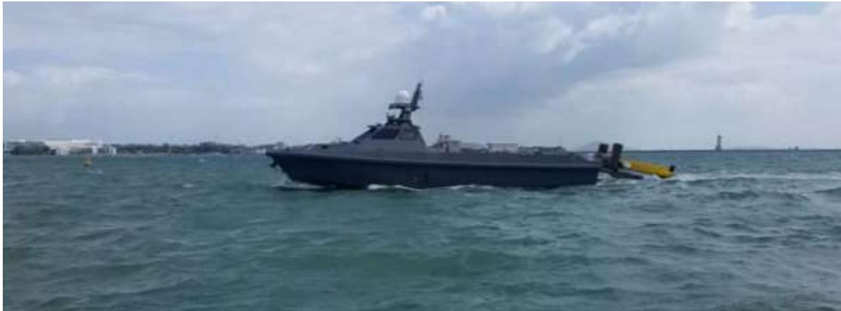
The Venus Unmanned Surface Vehicle (USV) is a modular USV designed to meet growing interest for configurable USV for multi-missions. The modular approach facilitates the integration of multi-mission modules to the USV which can then be configured for various missions without risking human lives.
