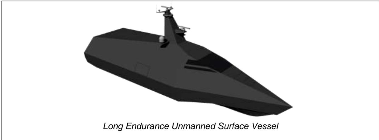
The Long Endurance USV (LEUSV) is designed to be a lightweight craft with high speed and endurance capability. The craft and the platform systems are operable and survivable at high sea state. The applications of the LEUSV are for anti-submarine warfare, maritime patrol and surveillance.
