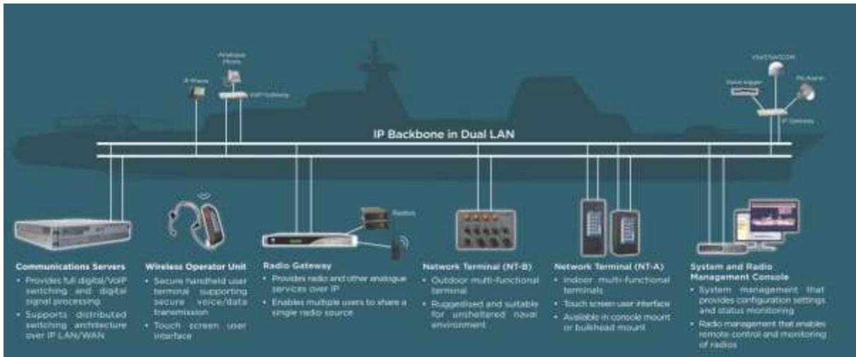
The SuperneT Shipboard Integrated Communications System (SICS) is a state-of-the-art Internet Protocol-based communications solution, designed and built for the mission-critical needs of today’s navies. The system integrates a variety of communications systems to offer feature-rich voice and data services that are easily accessible by users from fixed and wireless user terminals.
