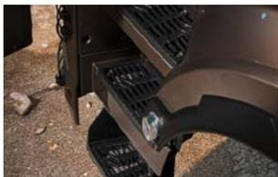
**The lowest step, which is prone to damage when driving off-road, is now movable. Its mounting brackets are made from flexible plastic, meaning that they can change shape if they come into contact with the ground and return to their original shape again afterwards.**
