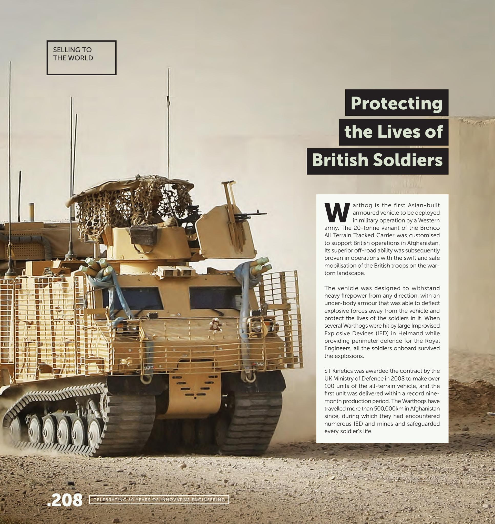
A Warthog tracked vehicle, a 20-tonne variant of the Bronco All Terrain Tracked Carrier, is shown in a desert environment. The vehicle is equipped with a turret, a machine gun, and various antennas. It has a protective cage around the front and sides. The background is a clear, bright sky.
