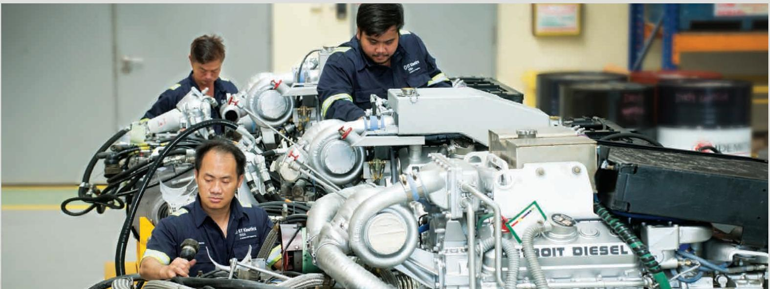
Bionix engine undergoing maintenance at ST Kinetics' component workshop.
