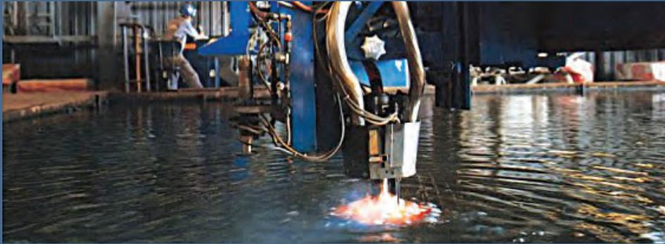
State-of-the-art underwater-plasma cutting machine installed in 1986.
