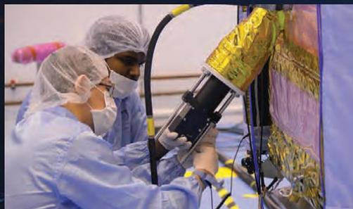
Engineers installing star trackers - primary attitude determination system - on TeLEOS-1.
