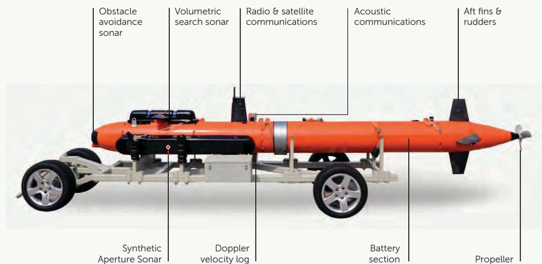
Mercury Autonomous Unmanned Vehicle
