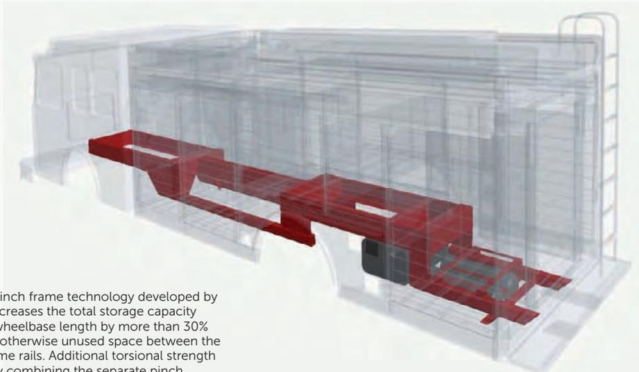
The drop/pinch frame technology developed by Hackney increases the total storage capacity in a given wheelbase length by more than 30% by utilising otherwise unused space between the original frame rails. Additional torsional strength is gained by combining the separate pinch and drop rails.
