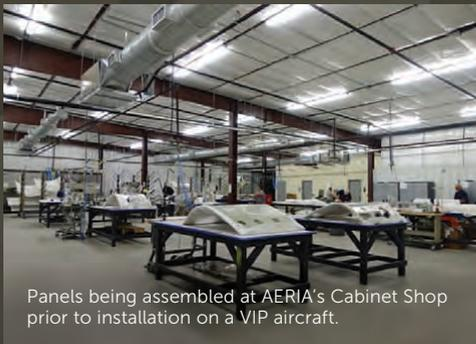
Panels being assembled at AERIA's Cabinet Shop prior to installation on a VIP aircraft.
