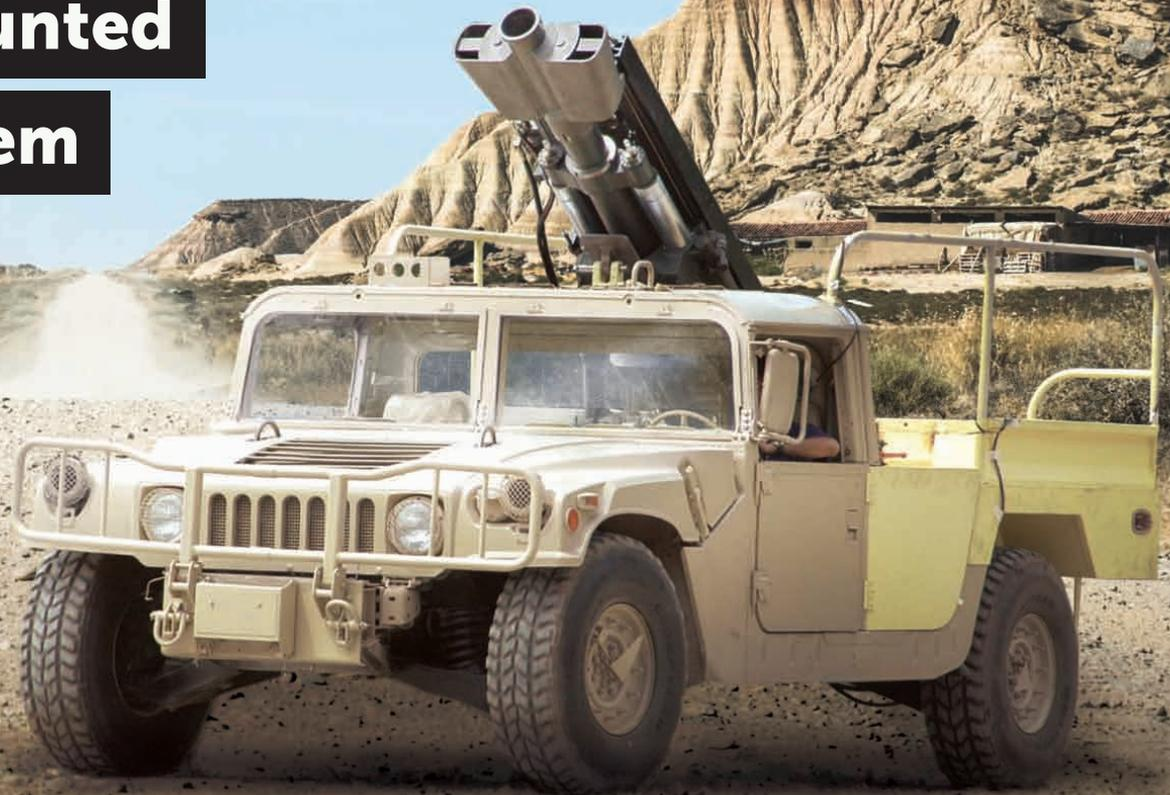
In 2004, Mr Teo Chew Kwee, Head of ST Kinetics' Weapon System Centre, proposed to develop a mortar system with a Middle Eastern partner. The system would comprise a 120mm Super Rapid Advanced Mortar Systems (SRAMS) and a fire control system mounted on a four-wheel drive light truck, to demonstrate the superior shoot-and-scoot capability of the combined system.
