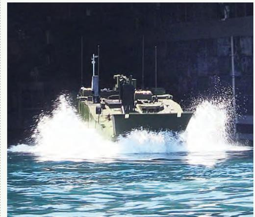
Terrex 2 launching from USS Somerset (LPD-25) in a launch-and-recovery operation trial in 2017.
