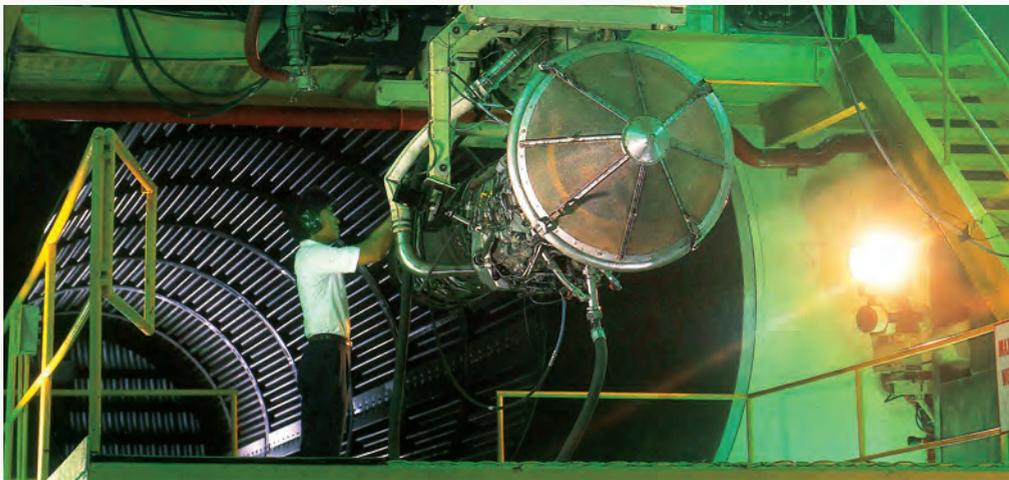
Rigging of a GE J85 engine for testing in the fully computerised test cell of Singapore Aerospace Engines, circa 1990.
