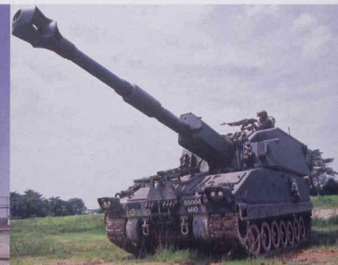
155mm howitzer, complete with digital fire control and programmable munitions magazine on board.
