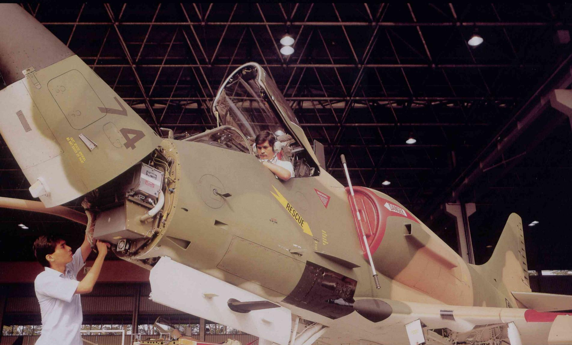
ST Aerospace upgraded the avionics of the A-4 with a state-of-the-art Weapons Delivery and Navigation System.
