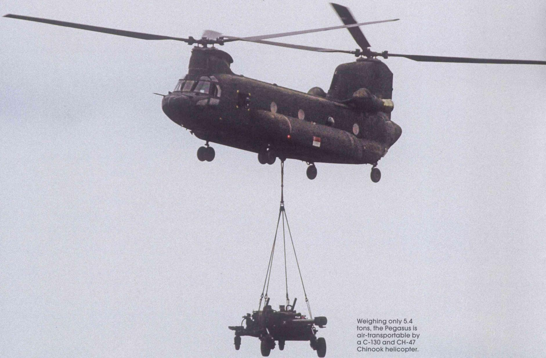
Weighing only 5.4 tons, the Pegasus is air-transportable by a C-130 and CH-47 Chinook helicopter.
