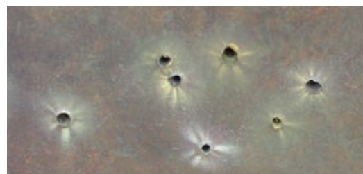
Penetrates 2.5" mild steel plate
